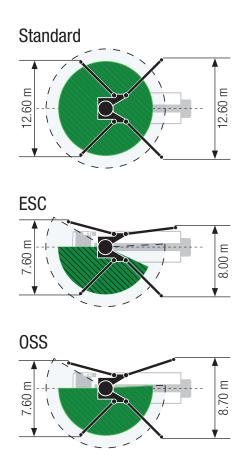
Support width based on center of support leg
