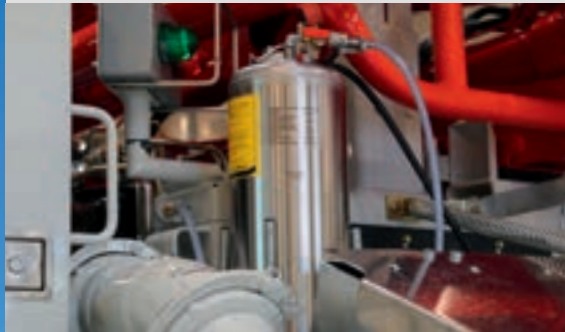
Spray tank with compressed air connection for easy cleaning of the hopper by moistening with release agent beforehand
