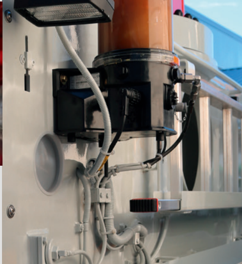
Spray tank with compressed air connection for easy cleaning of the hopper by moistening with release agent beforehand
